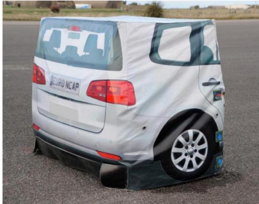
Figure 3: Euro NCAP Vehicle Target (EVT)
