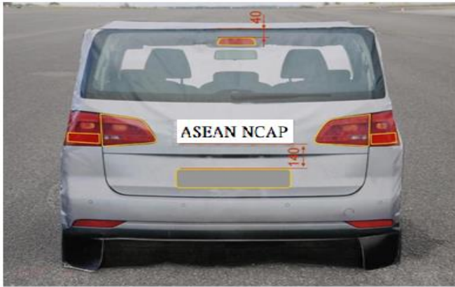
Figure A.2.1-1: Front view of the EVT with the location of the retro-reflective tape
