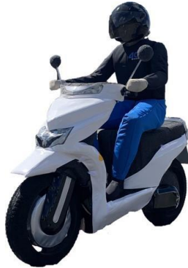
Figure 2: ASEAN NCAP Motorcyclist Target (AMT)
