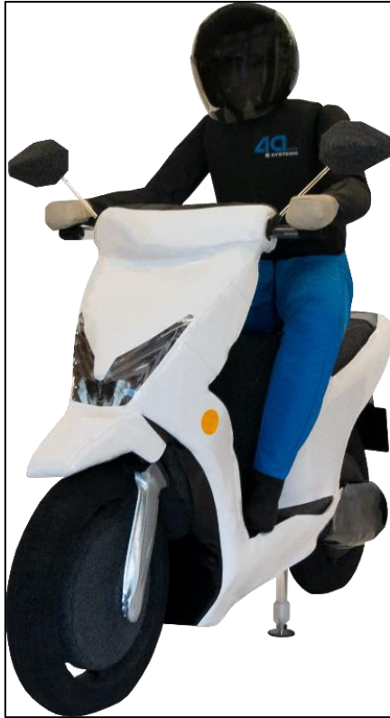
Figure A-1: Scooter rider and scooter target
