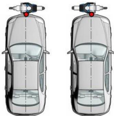
Figure 13: Impact points for CMCrossing test scenario
