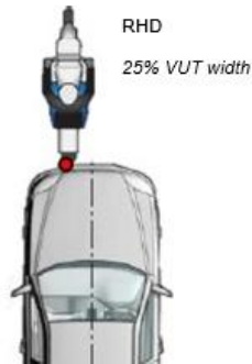
Figure 9: 25% impact point for CMRm scenario (FCW)
