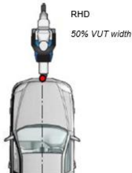
Figure 8: 50% impact point for CMRm scenario (AEB/FCW)
