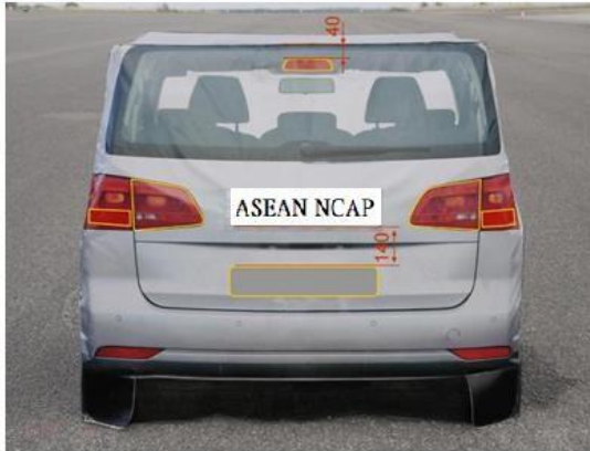
Figure A.2.1.1: Front view of the EVT with the location of the retro-reflective tape
