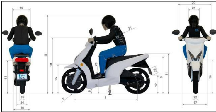
Figure A-2: Scooter target dimensions and dummy posture
