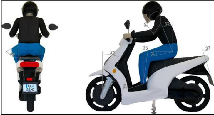
Figure A-3: Scooter target dimensions and dummy posture
